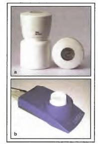
Fig. 1. Medication-Events-Monitoring System (MEMS®) device: (a) MEMS®V Smart Cap, with display showing that two doses have been taken; (b) MEMS® V Communication Device (photographs courtesy of AARDEX® Ltd./Aprex).
